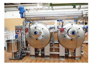
The SynthMaster operates by extremely low stretch and twist. Creases and rotation of the fabric are avoided thanks to plaiting device and the rectangular exit section of the plaiter arm.
