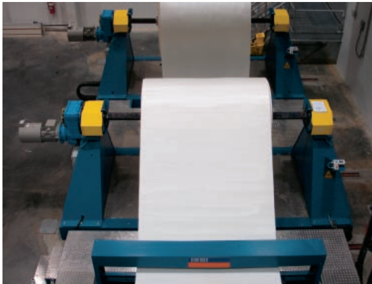
Dual centre driven Let-Off station with automatic fabric centring
