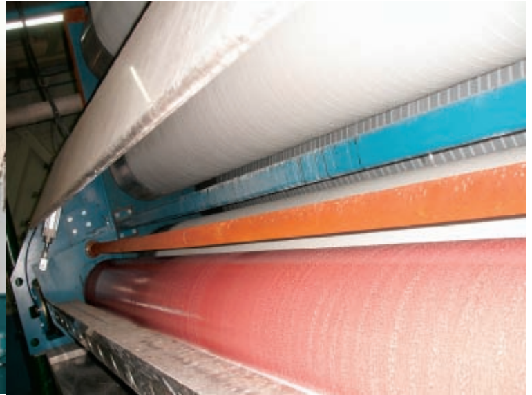
Scraper for cleaning the squeeze roll
