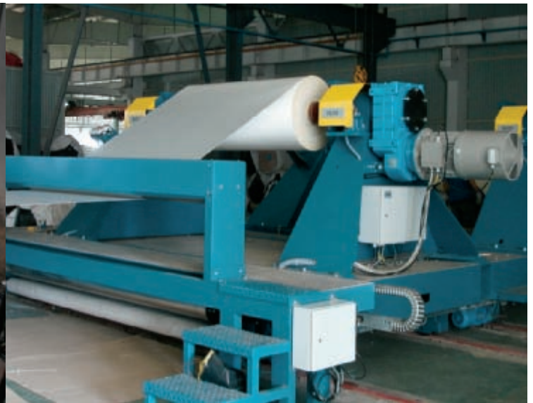
Dual centre driven Let-Off station with motorized drive
