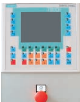
Operator panel (for each Let-Off and Wind-Up station)
