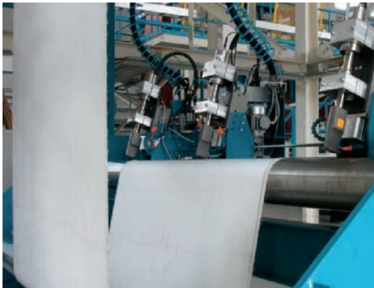
Cutting machine with 3 heads and automatic adjustment
