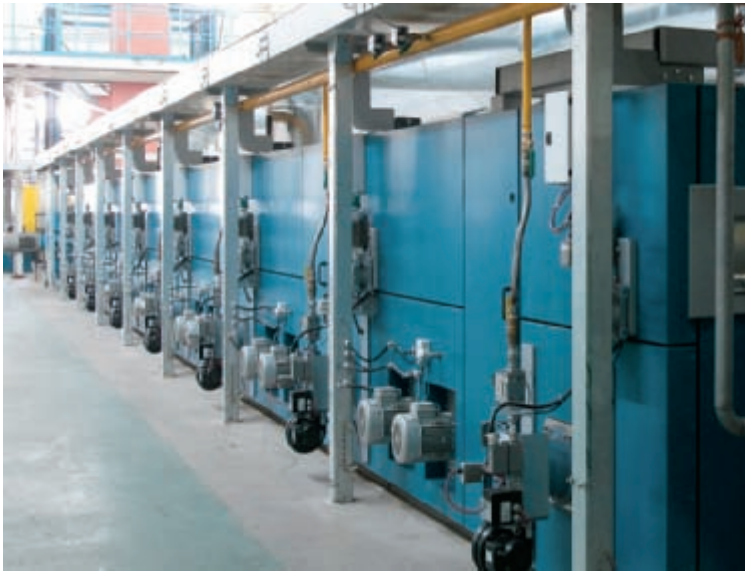
Stenter frame with 7 sections
