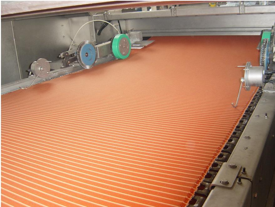
**Figure 2: BENNINGER: Conical inlet field where the fabric is pinned-on in the stretching field**
