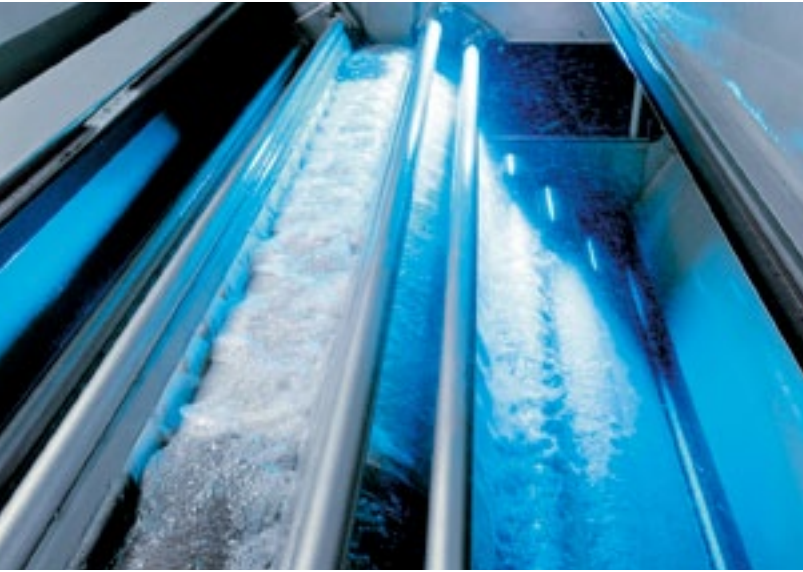
Open-width washing range for woven fabric
