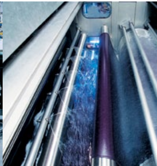
Open-width washing range for knitted fabrics
