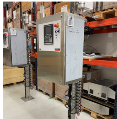
Chemical Dispensing System CDS
