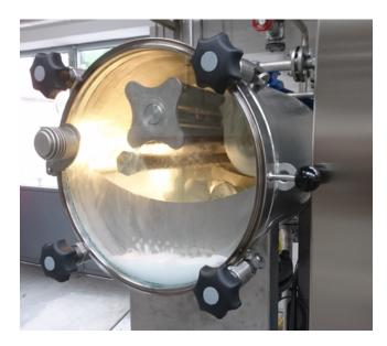
The machine is equipped with all features of a big machine namely, heating and cooling, filling, draining and rinsing.
