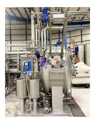
The machine distinguishes itself through an extremely compact construction – completely assembled with complete piping and wiring, the system can be connected and put into operation within a few hours.
