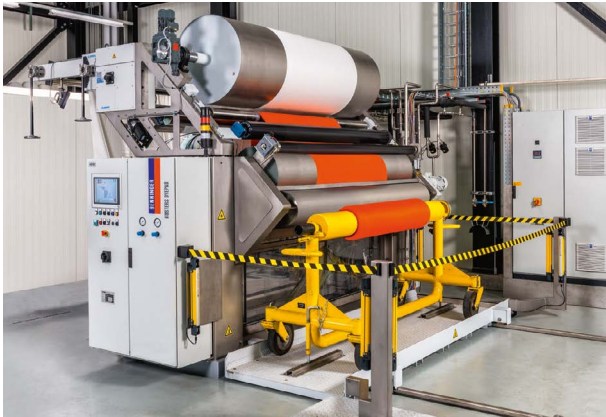
CPB dyeing station - dyeing at room temperature
